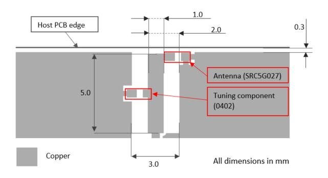
Below shows the PCB layout without solder mask for illustration purposes only.
